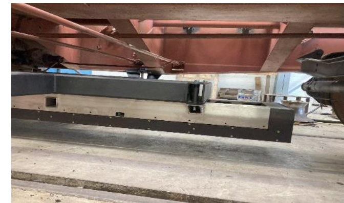
Figure 5 - Example of mounted mover magnet on conventional intermodal rail wagon (source NEVOMO)
